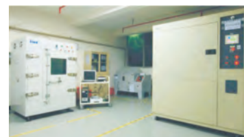
Natural convection test box (Left) Hot and cold impact test box (Right)
